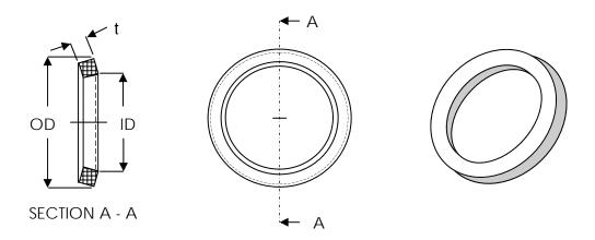
These preforms are designed specifically for SMP & SMPM series connectors. They provide optimum flow and fillet when used with the recommended preform well and are available in the following solders: Sn63, Sn96 or Sb5 for RACPO & RACMPO series and 80/20 Au/Sn for the RKCPO series.
